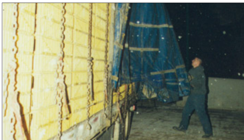
WRAPPED UP: Tarping chicken loads is now routine, but they don't always get the best airflow and ventilation during the summer and winter. A new prototype trailer in Saskatchewan may help fix this problem.
